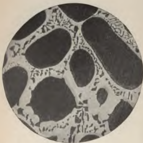
FIG. 16.—ALLOY OF SILVER AND COPPER— CU, 15% ; AG, 85%. Magnified 600 diameters.
